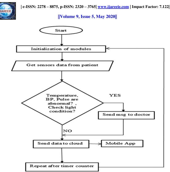
Fig. 5: Flow Diagram of the IoT based Smart Animal Health Monitoring System
