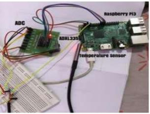
Fig. 3: Interfacing diagram of Temperature sensor and ADC with RPi3.
