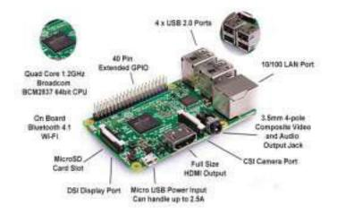
Fig. 2: Raspberry pi3 (top view)
